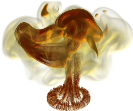
Figura: Volume rendered temperature data from the transient simulation of the 10-m heptane pool fire. http://www.sci.utah.edu/
