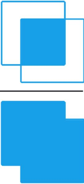
The diagram illustrates the IoU formula. The top part shows two overlapping squares. The intersection of the two squares is shaded blue. The bottom part shows the union of the two squares, which is the combined area of both squares, also shaded blue.
